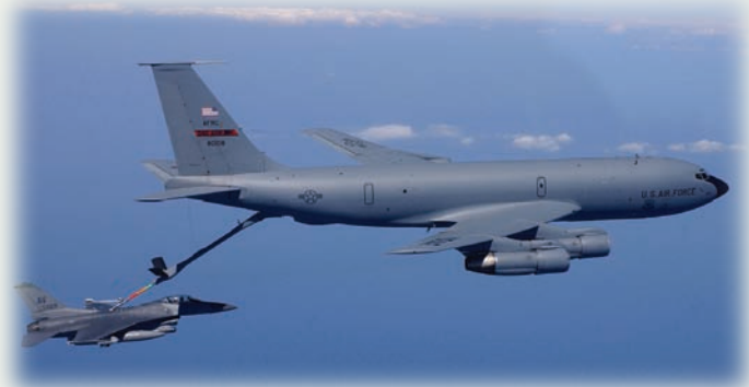
A KC-135 Stratotanker shown performing a mid-air refueling of an F-16 Fighter jet.
