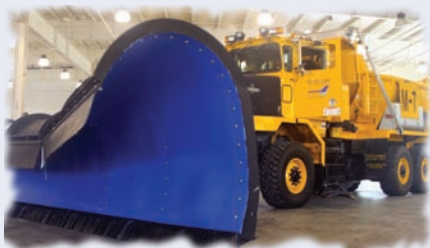
New to the GFIA fleet is this Oshkosh 6X6 P-series plow truck equipped with a 24-ft. Wausau gull wing plow.
